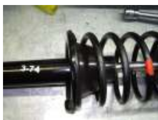
Strut markings from the factory
