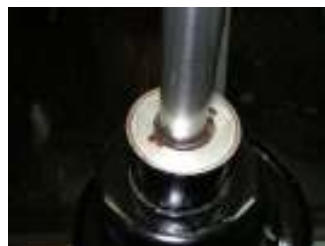
Strut shaft, seal & lock ring
