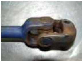
Intermediate steering shaft Uni Joint
