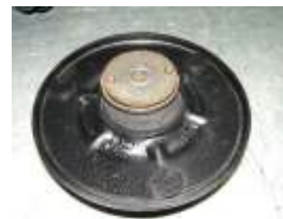
Bottom of Strut top with locating pegs
